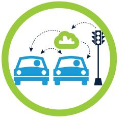
**Intelligent Traffic Management** regulates city traffic by using sensors and smart traffic signals to monitor, control, and respond to traffic conditions. Dynamic routing uses algorithms to proactively direct vehicles, determine optimal routes, and synchronize with other vehicles on the road. This reduces traffic and pollution while improving safety.
